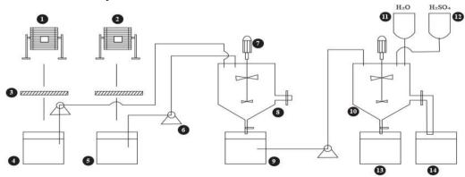
Fig: flow diagram of chrome recovery unit
